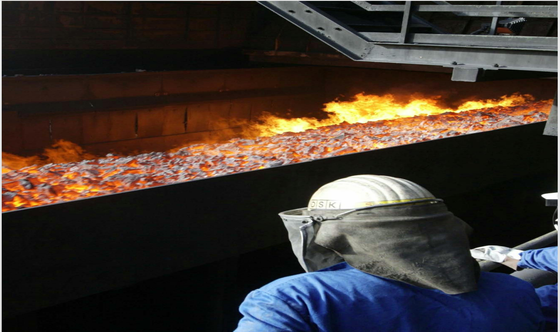
Coking Technology - Coke transfer
