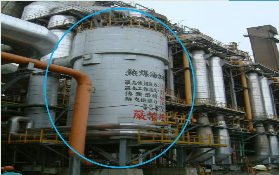
Ecoflow with thermal oil in steel industry at CSC Taiwan BF3, additionally with direct fired thermoil oil heater
