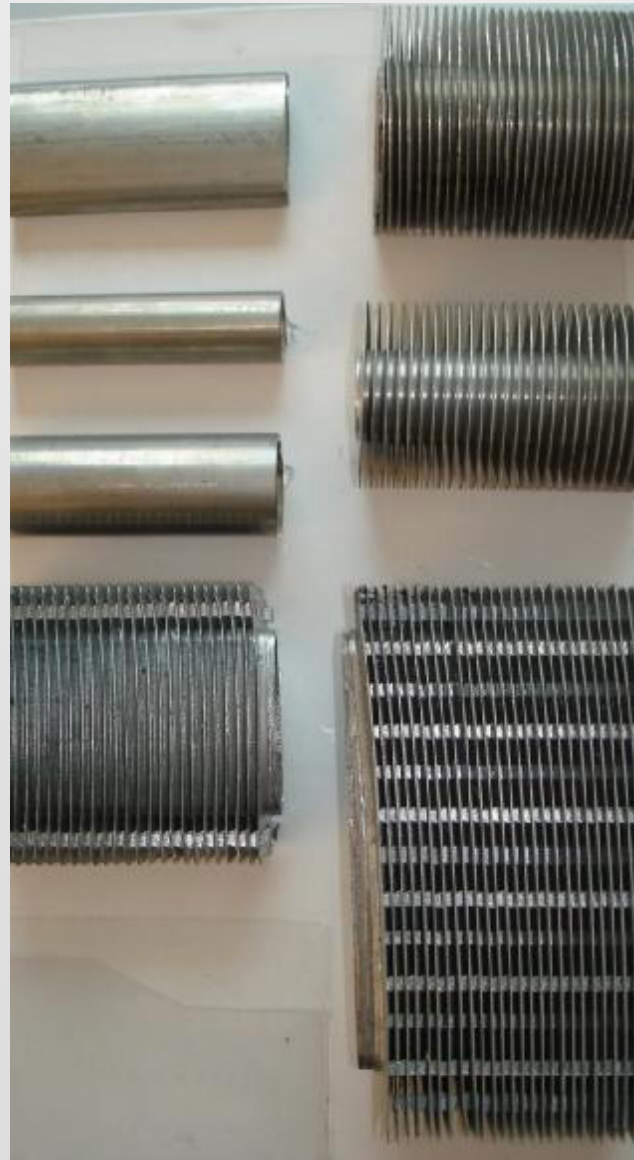
Heat exchanger pipe type round or oval resp. bare or finned
